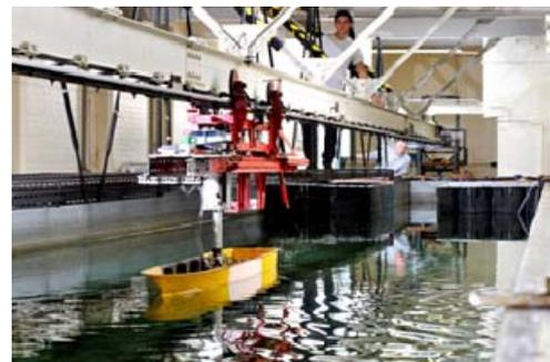
Figure1 Model Test in NEWU Towing Tank
