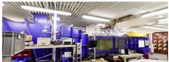
Fig.1 New Emerson Cavitation Tunnel
