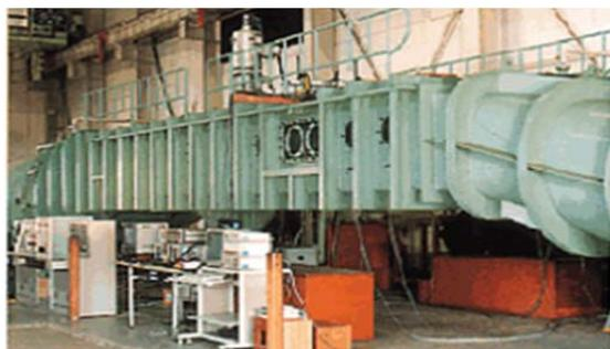
Fig.8 NMRI Large Cavitation Tunnel
