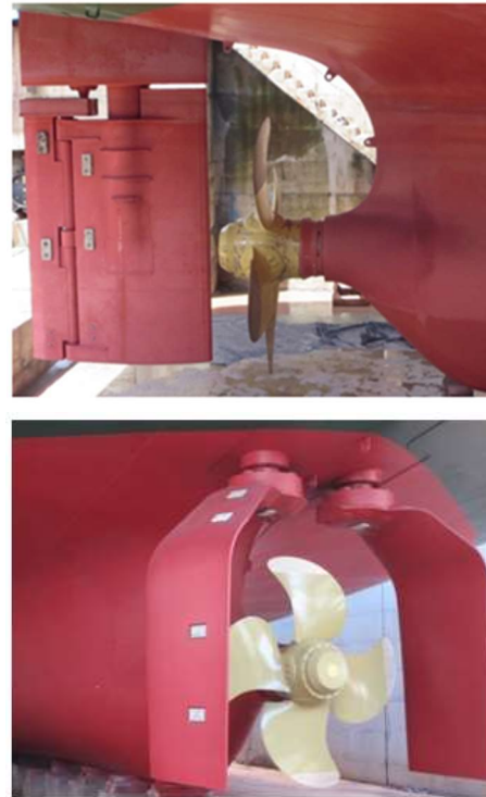
Figure 1. Conventional Flap-Rudder (Top) vs. GATE RUDDER® (Bottom)
