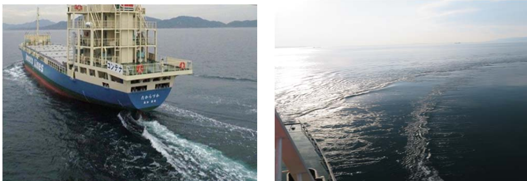
Fig. 24. Wave generation by conventional rudder (left) and low wake wash of GATE RUDDER (right)
