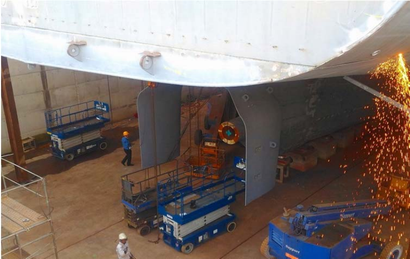
Fig. 2. Installation of GATE RUDDER on a container ship built by Yamanaka Ship Yard
