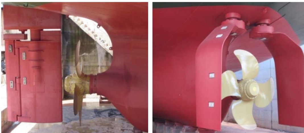
Fig. 8. Flap Rudder (Ship A) on the left and GATE RUDDER (Ship B) on the right
