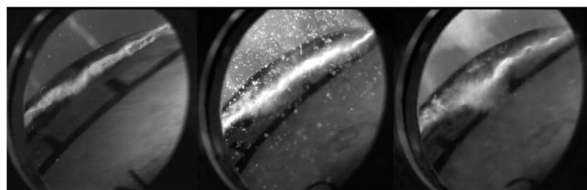
Figure 7. Comparative cavitation views about tip mid-chord region: Unmodified propeller (Left); Modified Propeller with less number of PressurePores™ (Middle); Modified Propeller with increased number of PressurePores™ (Right).
