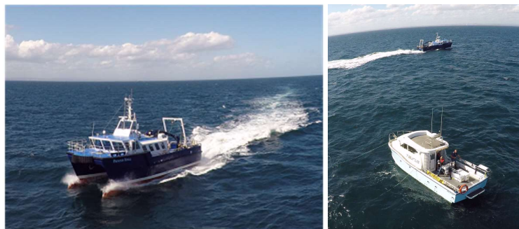
Figure 2. URN trials set up: Research vessel "The Princess Royal" passing by at full speed (Left); Support vessel deploying the hydrophone system with The Princess Royal passing at 100m CPA on the background (Right)
