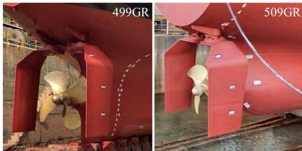
Fig.2 Installed GATE RUDDER with the same design on general cargo ships
