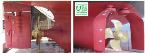
Fig.1 Flap rudder(left) and GATE RUDDER(right)
